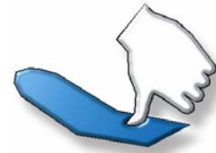
Be aware that tapes should be able to compress to allow the adhesive to make full contact with the receiving surface. Deep channels on the back of the glazing bars should be avoided as they could restrict full compression of the tape.
