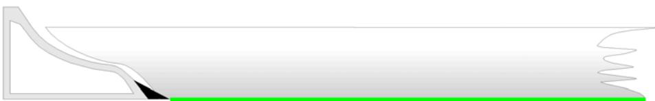
Here, the trim is being placed on the weatherseal, and as the bar expands, it moves up the sloping surface and a peel force is created and the tape releases from the glass.
