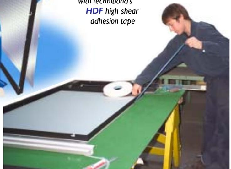
*Support frame and sheet being bonded with Technibond's **HDF** product. Once correctly aligned, the film liner can be slipped easily out from between the two surfaces, creating a long term permanent bond.*
